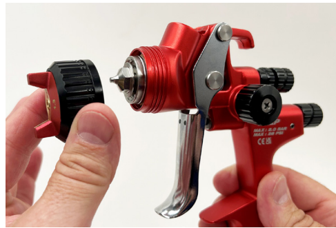
Remove air cap and thoroughly clean air cap (4) and nozzle (6).
